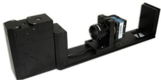
defects and measurements equal to a micrometer. A standard model supports an image field of 5 X 5 mm, accuracy up to 1 micrometer and resolution of 640 X 480. If you think this system sounds appropriate for your application, please consider speaking with one of our Engineers about it at 630-932-9380.
